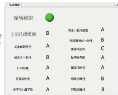
▲ To export to international companies, barcodes with grade B or above are required.
